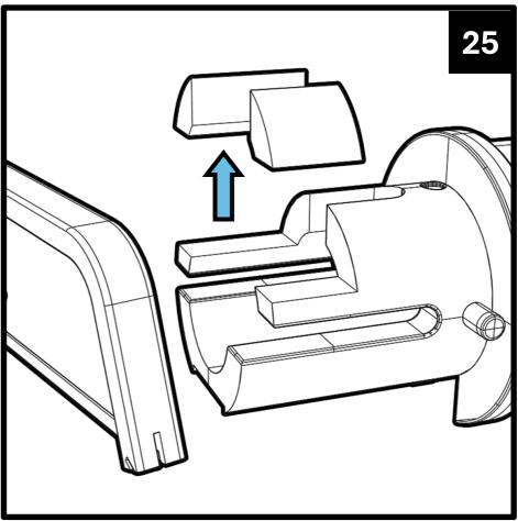
**26.** Combine the newly modified outer barrel with the G&G rotary hop-up chamber.
