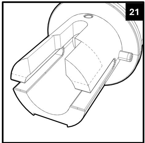
**22**. This is the what will look like for the left side of the outer barrel. The part inside the dotted lines will need to be removed.
