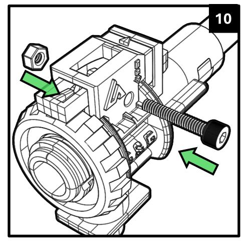
**11. Do not over lock the screw and nut.** A Firm lock will be sufficient.
