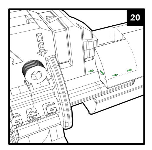
**21**. Once all dotted lines are connected you will get something like this in the demonstration pic for the right side of the outer barrel. The part inside the dotted lines will need to be removed.
