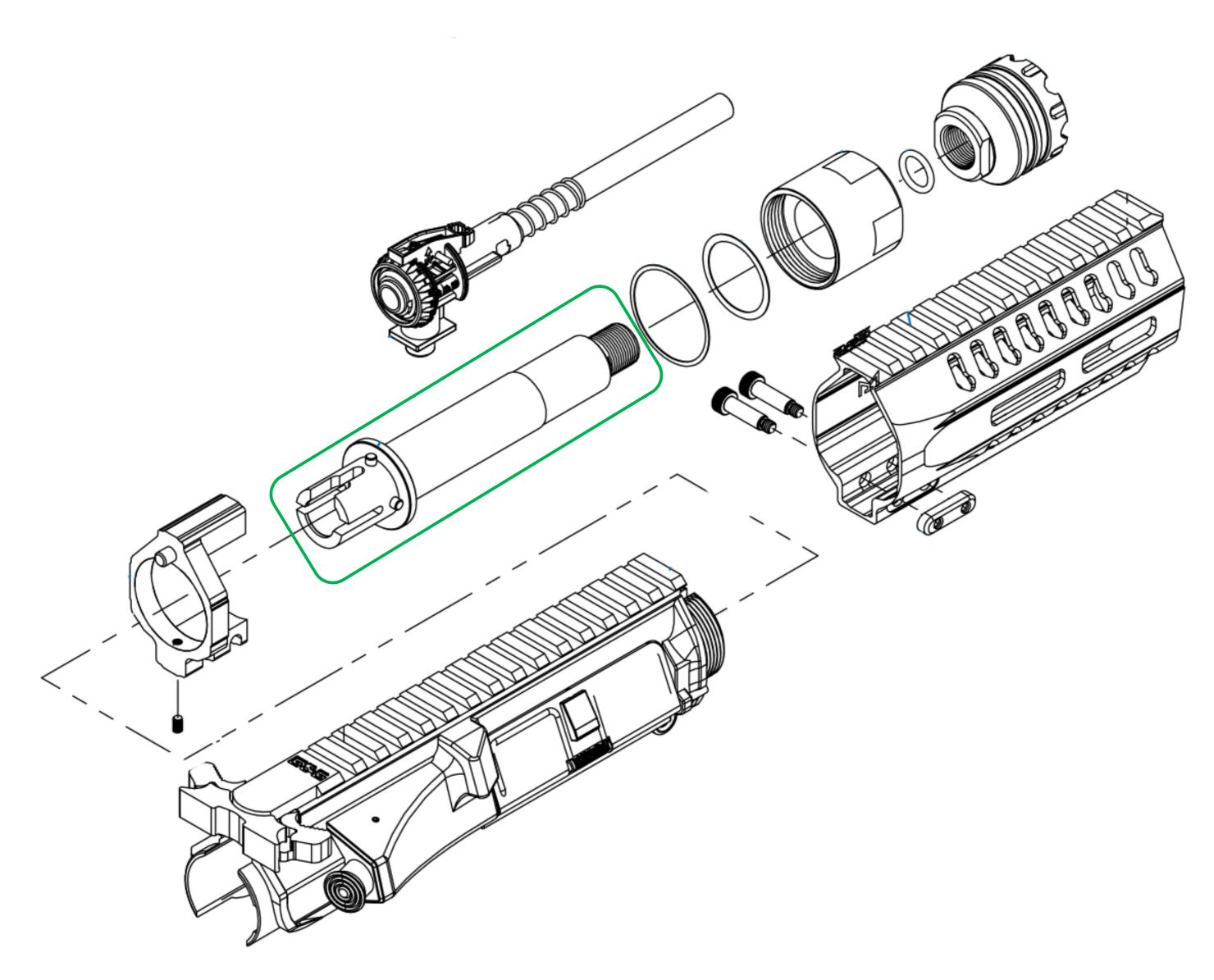
This section covers stage of separating and modifying the outer barrel in order for the TDC convertor to fit. The demonstration above shows a typical G&G CM16 upper receiver and the parts to take out to reach the outer barrel (highlighted in green). Above is the ARP9 model however much of the CM16 models are similar. This will let you extract the outer barrel for the next step.
