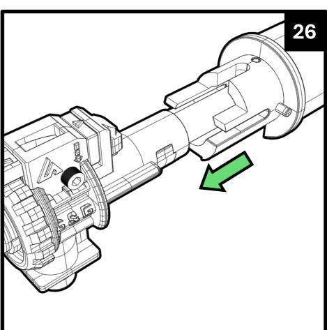
**27.** If don't correctly there will now be clearance on the outer barrel to make way for the upgraded G&G chamber.
