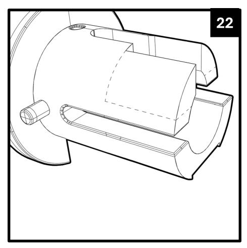
23. Cutting off the unwanted parts of the outer barrel.
